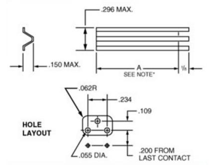
\* Note: "A" dimension may be specified from 0.25" minimum to 1.375" maximum in 0.125" increments
