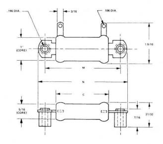
Standard oval resistors, like the miniature ovals, are easily stacked and utilize the mounting surface as a heat-sink. When stacking two or more parts the individual resistors should be de-rated as shown in the chart.
